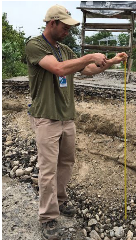
Aaron Gallant measures a down-dropped soil block through a road near the crest of the Petobo flowslide.
